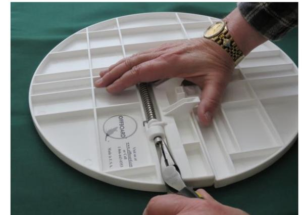
3) While pulling the bolt out, hold your hand over the spring so that as the bolt is withdrawn (You may want to use a glove over the spring at this point) so the spring does not fly off the door. **Retain the spring.**
